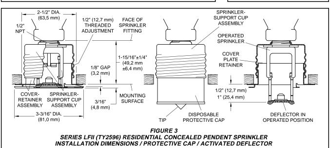
**Step 4.** Replace the Protective Cap by pushing it upwards until it bottoms out against the Support Cup. The Protective Cap helps prevent damage to the Deflector and Arms during ceiling installation and/or during application of the finish coating of the ceiling. It may also be used to locate the center of the clearance hole by gently pushing the ceiling material against the center point of the Cap.
