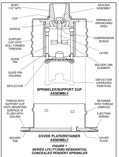
mum of 21 ft.lbs. (28,5 Nm) of torque is to be used to install sprinklers. Higher levels of torque may distort the sprinkler inlet with consequent leakage or impairment of the sprinkler.
